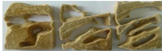
Fig.3 Photos of untreated Chinese fir samples attacked by termites
