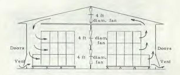
All material from this mill is air dried to 18 per cent. To improve drying a shed has been built in the air seasoning yard and as much stock as possible is dried under cover. The shed is 54 ft long, 36 ft wide and 13 ft high. It is divided into six bays 9 ft long. One bay has been enclosed to form a drying room and the sketch above gives a section through this room.
