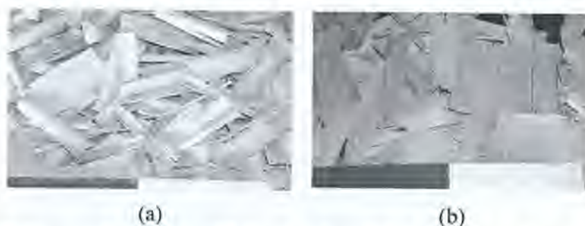
Figure 1: Examples of flakes produced from (a) green logs at room temperature and (b) logs conditioned at 70°C. White bar scale = 10 cm.
