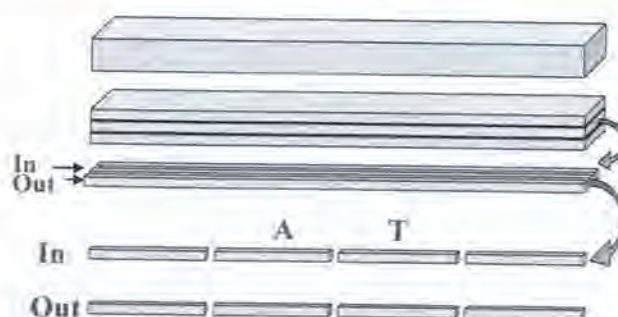
Figure 2: Cutting of specimens for various analyses
