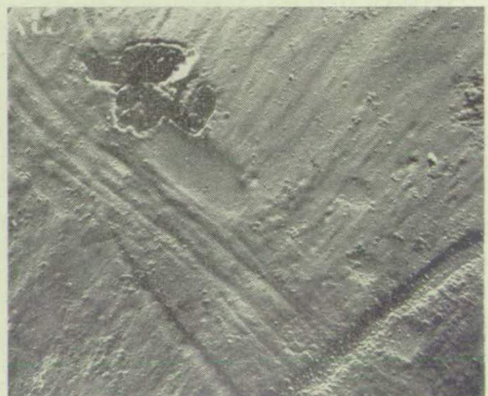
Fig. 5. Electron micrograph of a cell-wall of a tracheid with a fungally hypha and bacteria. (x 7200)
