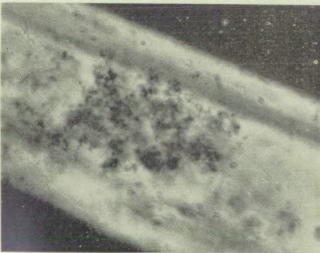
Fig. 4. Micro-organisms on the cell-wall of a tracheid. (x 1350)
