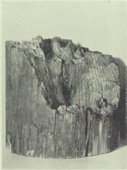
Fig. 2. Telegraph pole 8" in diameter, showing a brash fracture. Soft rot extended to the centre of the pole.
